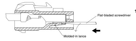
1. Refer to the drawing No. 1. Insert correct size screwdriver in the insulator against the molded-in lance. Deflect the lance as shown.
